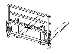
The Norden Euro Pallet Forks are an attachment that mounts to a loader or a tractor equipped with a loader having similar mounting capabilities. It is designed to move heavy pallet loads with ease.
