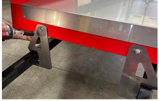
5. Remove Shipping brackets holding Chute in and remove the Chute.
