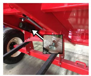
15. Place bolts into holes and tighten.
