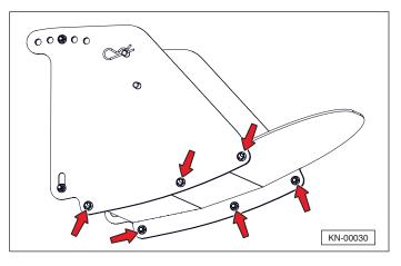
Loosely bolt the chamber extension onto the baler using four 3/8 x 1-1/4" carriage bolts and 3/8" flange nuts provided. Make sure the carriage bolt heads are on the inside.
