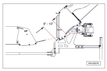
6. Ensure that the belt tensioner assembly is square with the belt by adjusting the angle of the belt tensioner assembly at its mounting point on the base chute.
