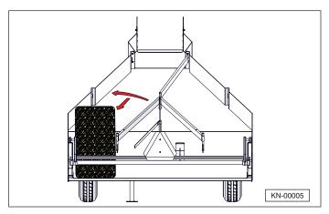
Bale #2 enters the Hay Accumulator and slides downward and into position, rotating the gate flipper and shifting the center gate to open row #3.
