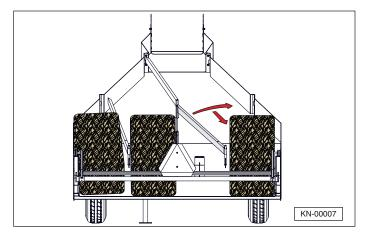
4. Bale #4 enters the Hay Accumulator and slides downward. As it slides into position, it depresses the back gate paddle, releasing the gate.
