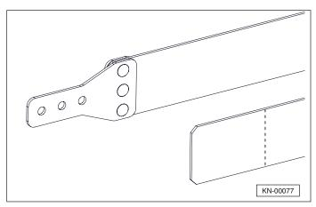
10. Using the small end plate as a guide, drill three 7/16" holes through the belt. Remove the excess length.
