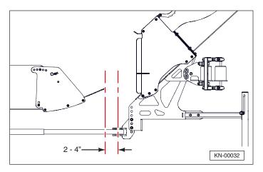
5. Select one of the five holes on the adjustable bale chamber extension that will best guide the bales into the Hay Accumulator base chute.
