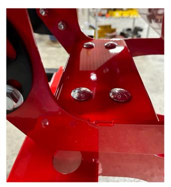
11. The top of the chute is fastened to the accumulator with two 3/8" x 1" Carriage bolts. Use an alignment tool to position the chute and bed to allow placement of first bolt.
