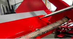
12. Place bolts into holes. You can tighten these right away.
