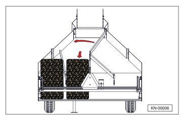
3. Bale #3 enters the Hay Accumulator and slides downward and into position, rotating the right gate to open row #4.
