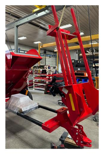
9. Set the chute assembly onto the frame, line up the bolt holes at the bottom.
