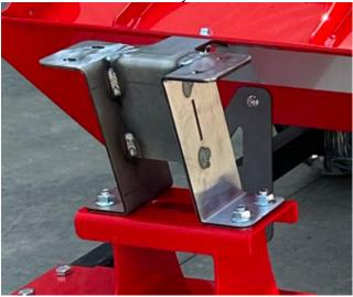
4. Remove the shipping brackets holding the front of the bed to the reach poles.
