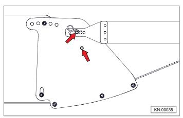
8. Use pin for setting up belt length. Remove pin after belt is cut to proper length.
