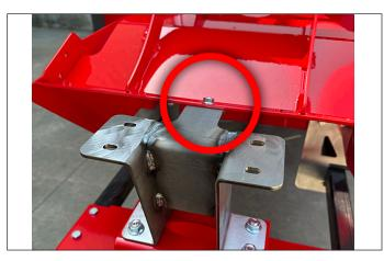
3. Remove bracket from the chute mounting plate. Keep the bolts handy as they will be used to fasten the chute assembly.
