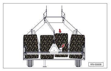
5. Once the back gate is open, the bales drop to the ground. When all bales are clear, the back gate returns to its original position and latches. All gates return to their original position.
