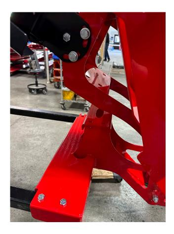
10. Place four 1/2" x 1" Carriage bolts into the chute, fastening it onto the frame. Install the flange nuts but do not tighten nuts until after the top bolts are also in place.
