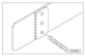
11. Install the belt end plates using three 3/8 x 1" carriage bolts and flange nuts. Position the large end plate on the inside (nearest to the bale chamber).
