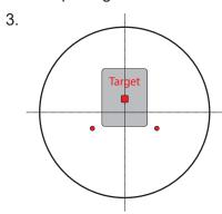
Drive the spear into the bale with the spear level, centered horizontally, and the point of the spear at, or slightly above, the vertical center of the bale, until the spear is fully inserted and the bale is against the bale spear frame.
